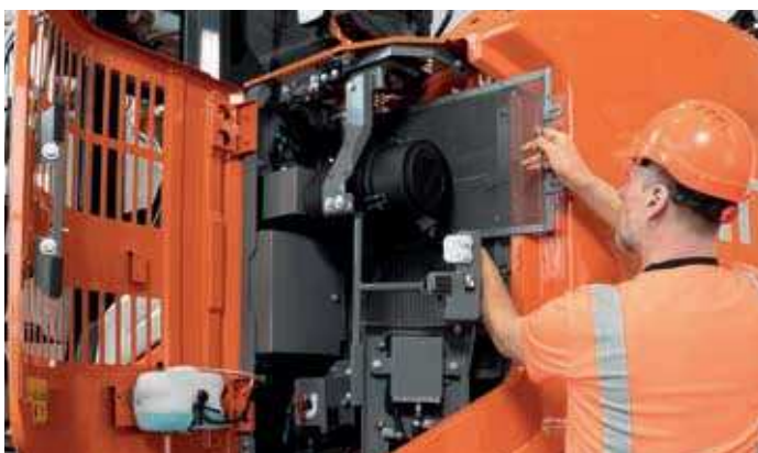
Enlarged radiator door (ZX135US-7) provides easy access for cleaning and maintenance.
