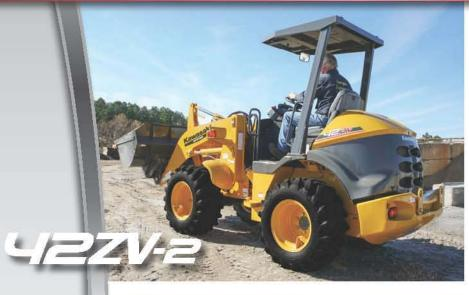
Wrap-around counterweight lowers the center of gravity increasing stability Universal Quick Coupler allows a wide range of attachments Interchangeable with skid steer
