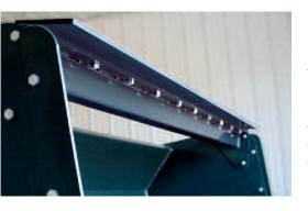
Optional "Pull-Back" system for increased versatility. Helps pull back snow from tight spaces. Ideal for curbs, overhead doors, loading docks, and against buildings.
